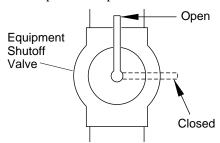
Figure 16 - Equipment Shutoff Valve
